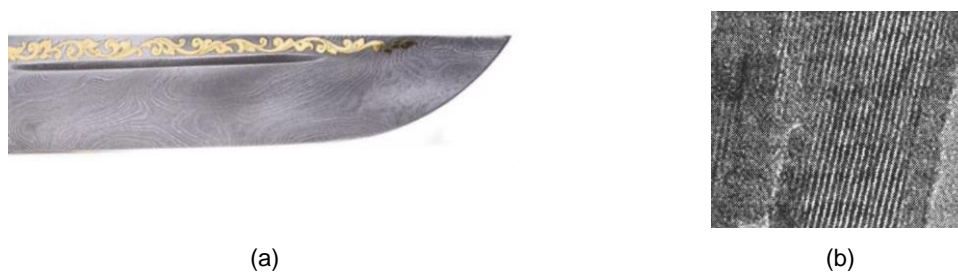
Fig. 2. (a) – Damascus steel sword and (b) - Damascus steel nanostructure
