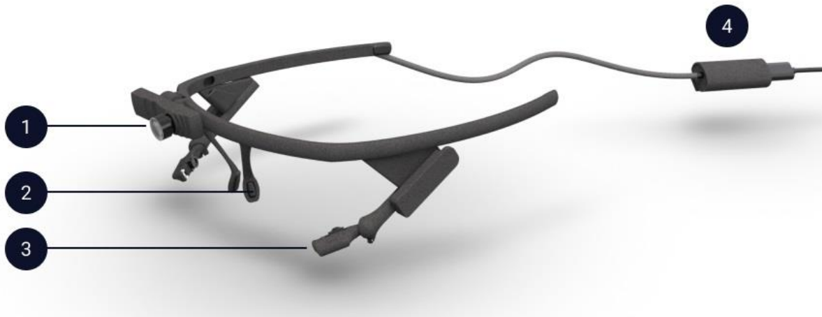
Fig. 1. Pupil Labs Core binocular headset: 1) world camera; 2) nose grip; 3) near infrared camera; 4) USB-C interface
