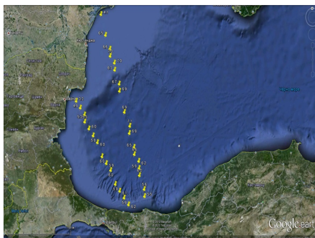
Fig. 11. Right track-SWH (m), measured by ENVISAT satellite on 07/02/2012, 21UTC and left track-SWH from JASON1 on 08/02/2012
