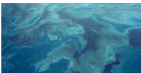
Fig.1. Scattered patches of heavy fuel oil spreading to brown and silver sheen in warm ambient conditions (air temp \sim 30^{\circ}\text{C} , water temp \sim 25^{\circ}\text{C} ). Viewed from 300 m
